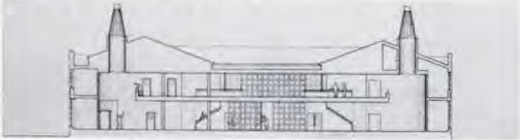
section B-B through bridge showing two-storey voids and conical skylight lanterns over entrances; sliding panels in centre are earlier design
