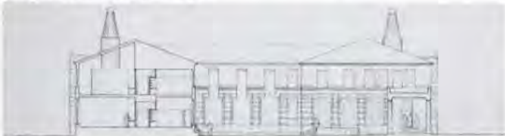
section C-C through new wing showing preferred part of studios, off-centre corridor and offices facing court; elevation of existing building shown with intended 'bottle windows' on two-storey gallery facade
